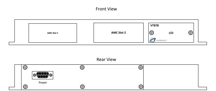
Figure 3: VT878 Chassis Layout
